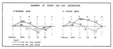
The results of measuring a kiln twice, first cold and then after a short interval, hot, is shown in this chart. The shell axis is shown in both the horizontal and vertical planes to support the contention that measuring a kiln in a static condition does not provide sufficient accuracy for optimum adjustments.
